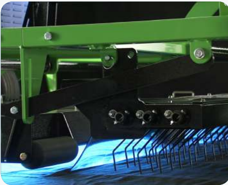
The spring tine rake attachment is equipment with 42 tines that comb through the turf surface, lifting fiber and infill, preparing the turf for exposure.
