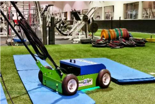
The spring tine rake attachment is equipment with 42 tines that comb through the turf surface, lifting fiber and infill, preparing the turf for exposure.
